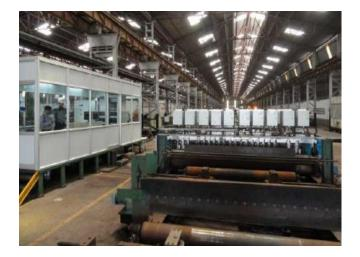
The Coil/Plate test systems is to test the lamination defcets parallel to the surface based on the International Standard ASTM-SA 435, API & similar specification. The Test Mechnism will have probe boom having probe arrangement to scan grid scanning (selectable), 100% scanning or 100 % with specified overlap say 10%.
